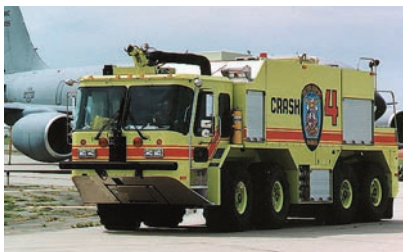
One of the airport rescue and firefighting vehicles available. This vehicle carries 3,300 gallons of water and 500 gallons of foam.
